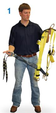
1 Grasp harness by back D-ring and back plaque. Be certain straps are not twisted, and inspect for damage.
