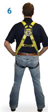
6 Back D-ring should be centered between shoulder blades. To adjust, slide D-ring and plaque up or down along the webbing.
