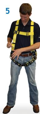
5 To tighten shoulders, pull up on free ends of straps. To loosen, push down on adjuster. Straps should be adjusted to the same length.
