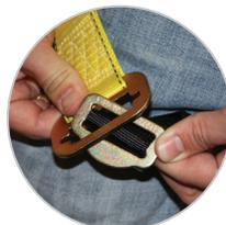
Pass-Thru buckles are zinc-coated and smooth for a precise fit. Placement of the web through the buckle provides for a higher degree of custom adjustment than grommet and tongue buckle fasteners, and use of Pass-Thru buckles reduce the overall weight of the harness. Pass-Thru buckles are standard chest strap fasteners on all Reliance harnesses.
