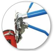
Anchor ring installation on an irregular shaped tool utilizing the 799990 tool. Consult instruction manual for use and installation details.
