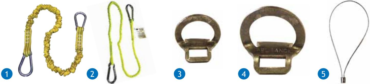
**799955 Tool Lanyard:** (Fig.1) Lanyard is designed to arrest dropped tools weighing up to 50 lbs (23kg). Lanyard is elasticized and contains an energy absorber that limits forces to 450 lbs (2 kN). Includes spring hooks on each end.
