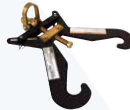
Lockjaw™ Beam Grip 3040 Attaches to I-beams 5"-12". Aluminum jaws, steel swivel. 10k lb anchor point.
