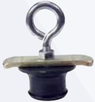
Metal Decking Insert 2243 Attaches receiver to 2" holes in decking. Eyebolt used to remove insert after pouring. 2241: Urethane insert only.
