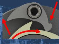
2. The continued rotation and spring pressure lift the pawl away from the sperrad locking tooth.
