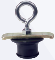
Metal Decking Insert 2243 Attaches receiver to 2" holes in decking. Eyebolt used to remove insert after pouring. 2241: Urethane insert only.
