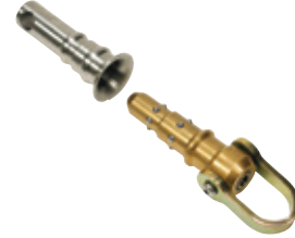
Concrete Embed Anchor 2250/2252/2260 Carbon (2250) or stainless steel (2252). Provides up to 10,000 lb. anchor when attached to receiver. May be used for one or two man anchor or to anchor horizontal lifelines.
