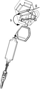
**4.** Slide the open end of the carabiner into the webbing loop (g) and rotate until the gate is down (h).
