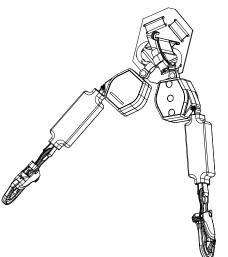
**6.** Ensure that the carabiner gate is in the fully locked position and that the carabiner lock arms are fully snapped onto the carabiner.
