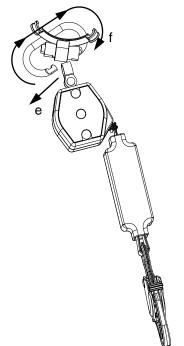
**3.** Slide the open end of the carabiner onto the top swivel of the first SRL (e). Slide the SRL all the way around to the backside of the carabiner (f).
