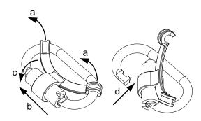
2. Lift the arms of the carabiner lock up (a), unlock and open the carabiner by pushing the gate forward (b), rotating the gate (c) and pushing the gate in (d).
